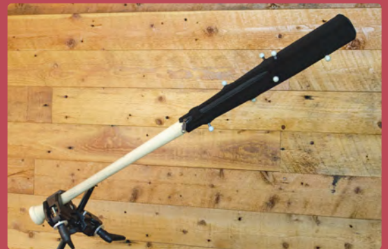
Custom motion capture controller for VR baseball experience.
